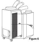
An ambient air adapter can be purchased separately. Air adapter fits over the condenser to duct condenser air to the unit to improve cooling efficiency. 1.Remove air adapter from carton.
