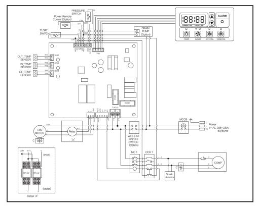
Figure 11 - Circuit Wiring Diagram
